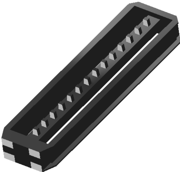
Illustration 18: Model of a Weber Reference Bar.
